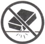
Handle the metal detector gently and carefully. Dropping it can damage circuit boards and cases and can cause the metal detector to work improperly.
