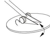
2. Tighten the knobs so that it is just enough to keep the search coil from rotating or wobbling.
