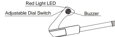
2. Hold the search coil level and about 1-2 inches above the ground, slowly move the search coil over the ground, sweeping the search coil in a side-to-side motion.
